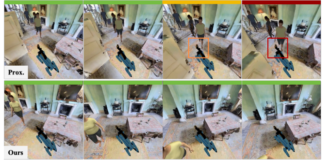
(c) Frontal Approach: The Proximity-Aware method collides when crossing in front directly, while our method avoids safely by anticipating human path.
