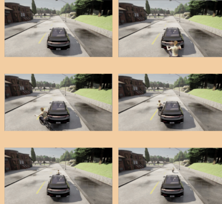
Figure 2: Example ScenicNL output and its respective CARLA simulator visualization. The natural language description was parsed from a California DMV Crash report. It specifies the collision between a cyclist and paused autonomous vehicle.
