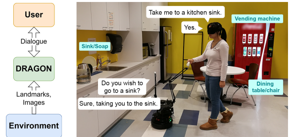
Fig. 1: DRAGON identifies the intents of the user through dialogue, grounds language with the environment, and guides the user to their desired goal.
