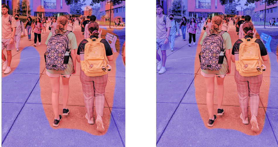
Figure 1: An illustrative example of the difference between attentive regions from computer vision models (left) and navigation models (right). With the assumption that everyone respects social etiquette, some regions become redundant when making navigational decisions.
