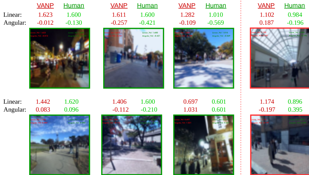
Figure 4: VANP’s qualitative performance on unseen scenarios. Green: VANP outputs align with the demonstrations; Red: VANP outputs do not align with the demonstrations.
