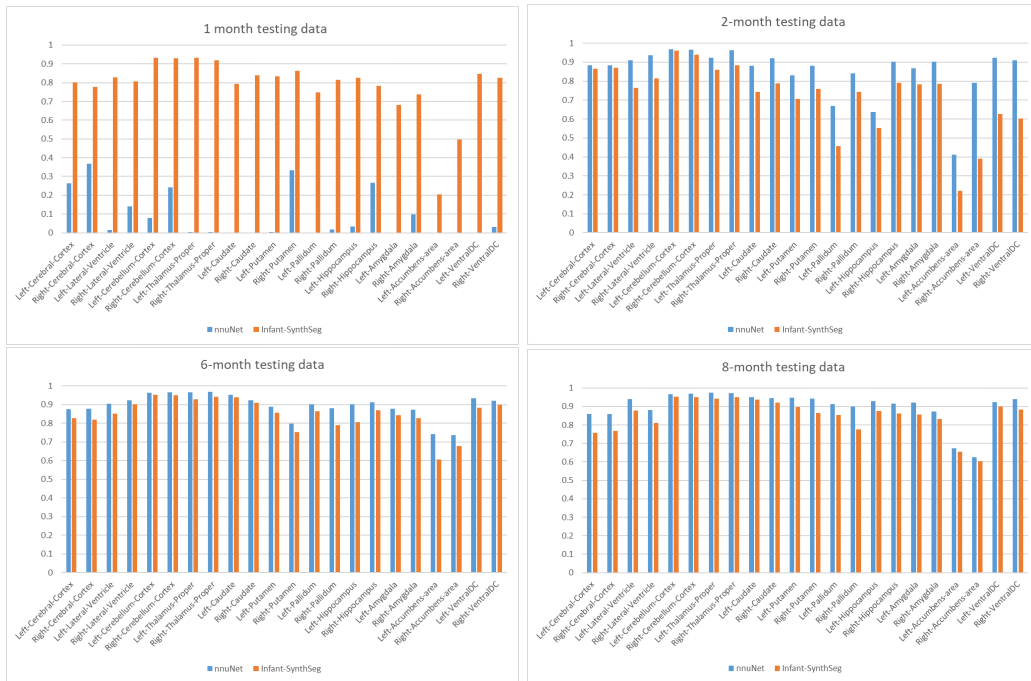
Figure 4: Dice score: SynthSeg-infant (SynthS) vs nnU-Net (NNU), each 1 subject at 1, 2, 6, 8 months. While nn-UNet fails at 1 month, it overall performs at a similar or better level for the other ages.
