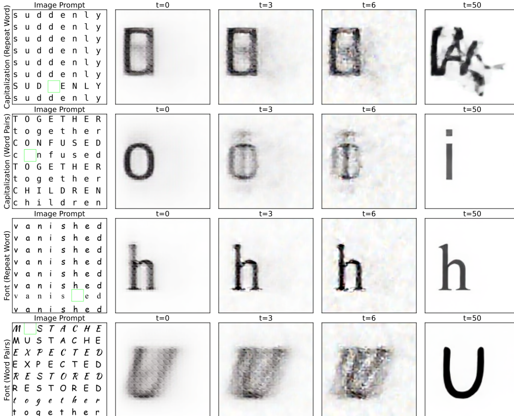
Figure 3: \hat{x}_0 visualization [7] of character inpainting across timesteps, where t = 0 indicates the first timestep and t = 49 is the final output. FLUX.1-Fill is often correct at the first timestep, but after subsequent iterations it sometimes “changes its mind.” For example, the bottom row shows that the model is beginning to correctly inpaint a Kaushan Script ‘U’, which is later incorrectly replaced by a verbatim copy of the adjacent Comic Sans ‘U’.
