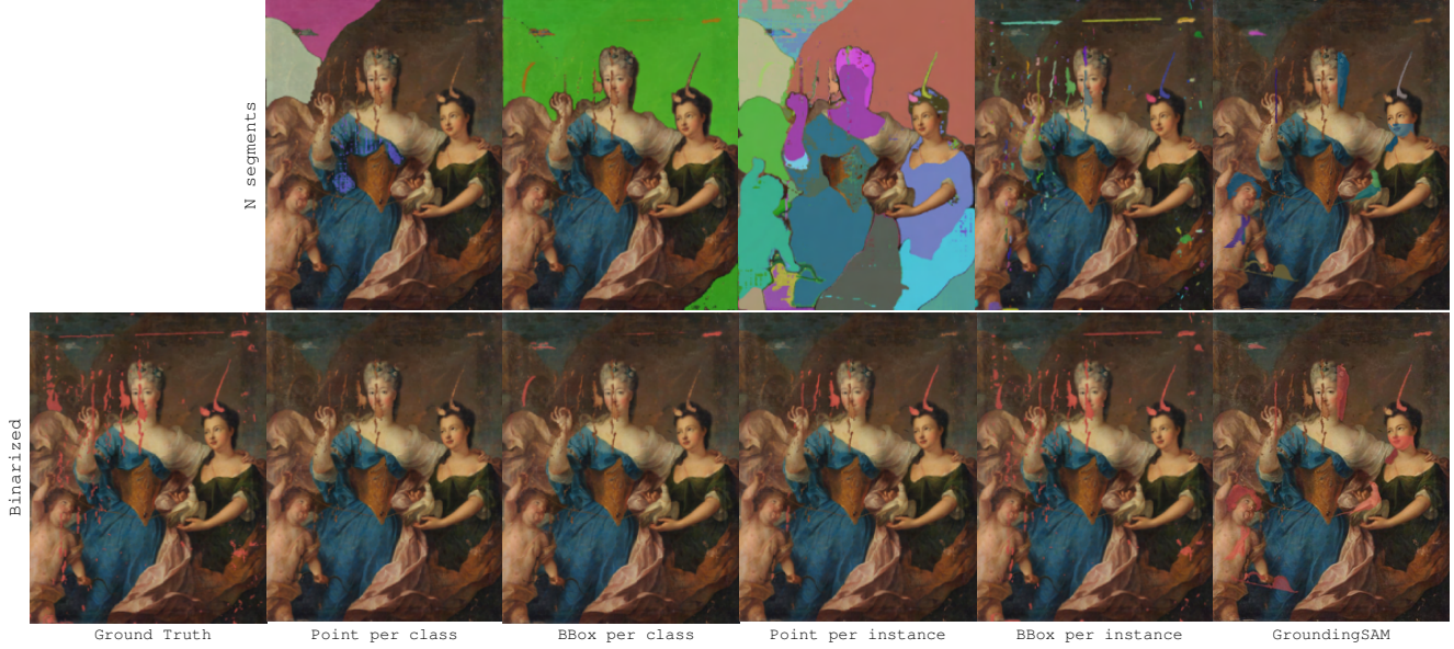
Figure 4. Qualitative results for SAM at zero-shot damage segmentation. Top row shows initial segments from N prompts as predicted by SAM (unique colour per prompt), bottom row shows the segments after being assigned binary class (Clean or Damaged) via an oracle.
