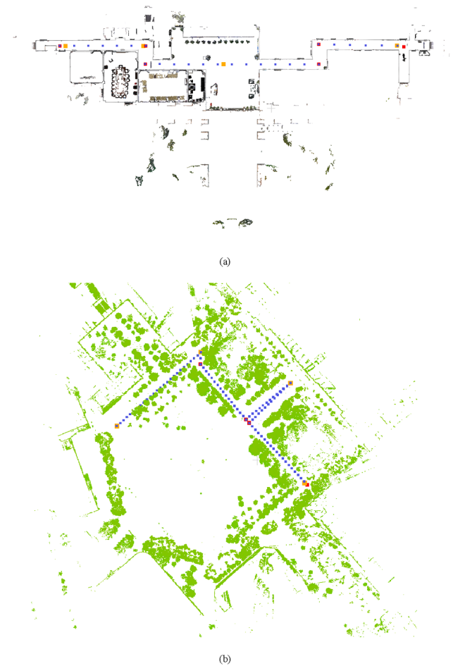
Fig. 19. The locations of real scans, virtual scans, and control points. In the figure, the blue point is the location of the virtual scan; the red point is the location of the picked control point; the origin is the location of the real scan. To display the location more clearly, the points of ground and roof are removed in the indoor scene and the points of ground are removed in the outdoor scene. (a) A top view of the 3D map of the indoor scene; (b) top view of the 3D map of the outdoor scene. (For interpretation of the references to colour in this figure legend, the reader is referred to the web version of this article.)
