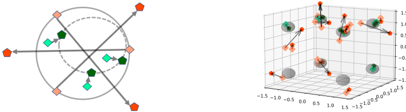
Figure 5: A depiction of why collapsing happens. Left: An illustration. Right: Experimental observations on the 3-dimensional Gaussian mixture dataset. In the illustration, the original particles (orange rhombi) near the boundary of the mode (solid gray circle / sphere) will be pushed to a significant distance (orange-red pentagons). The particles within the mode (green rhombi) will stay close to their original places (dark green pentagons). This contracts the boundary of the mode (gray dotted line).
