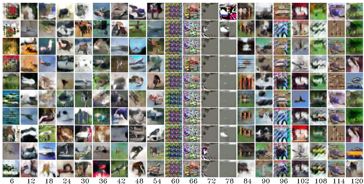
Figure 35: Generated images in trial 2. The stopping point is the 68th epoch. Before the stopping point, the generated samples demonstrate good quality, particularly evident around the 54th epoch. Approaching the stopping point, they become contaminated by noise. Afterwards, they regain clarity, but transition between different modes.
