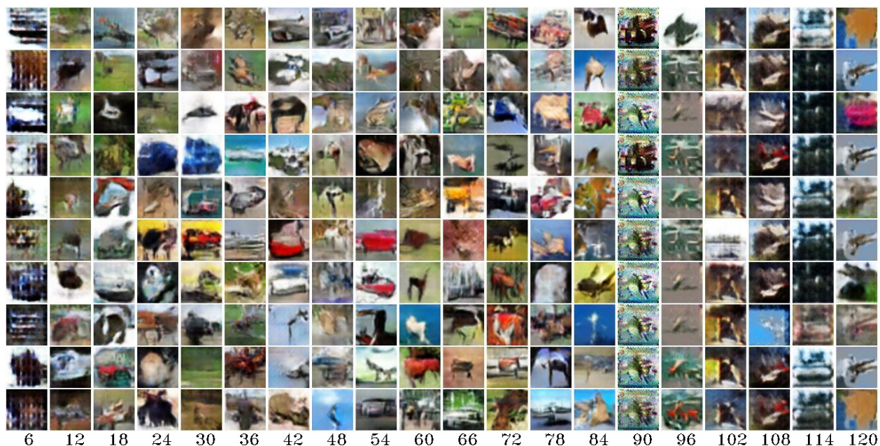
Figure 34: Generated images in trial 1. The stopping point is the 93rd epoch. Before the stopping point, the generated samples demonstrate good quality, particularly evident around the 78th epoch. Shortly after surpassing this point, they become contaminated by noise. Afterwards, they regain clarity, but transition between different modes.
