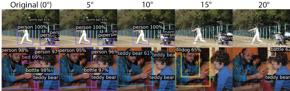
Figure 1: The COCO-Periph Dataset contains MS-COCO images that have been transformed to visualize the loss of information in human peripheral vision due to visual crowding (not just acuity loss) at various eccentricities. This loss of visual information causes difficulties for computer vision systems: models such as Faster-RCNN (shown here) perform poorly at tasks like object detection as simulated eccentricity increases. In contrast, human performance is known to fail gracefully, raising the question: how can we close this gap?
