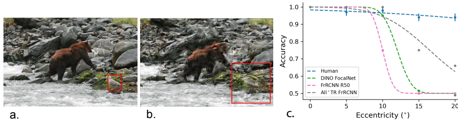
Figure 3: Example Easy Object Detection. (a) Original image with target object bounding box, and (b) TTM transform for 15° (240 pixels) with extended bounding box (used to perform machine object detection task). (c) Human accuracy for peripheral viewing of example image averaged over all subjects with error bars reporting SEM (blue), compared with accuracy on TTM image for a pre-trained (pink) and trained on COCO-Periph (gray) Faster RCNN R50 model, and a DINO FocalNet model (green). Psychometric curves are fit with an inverse cumulative normal distribution.
