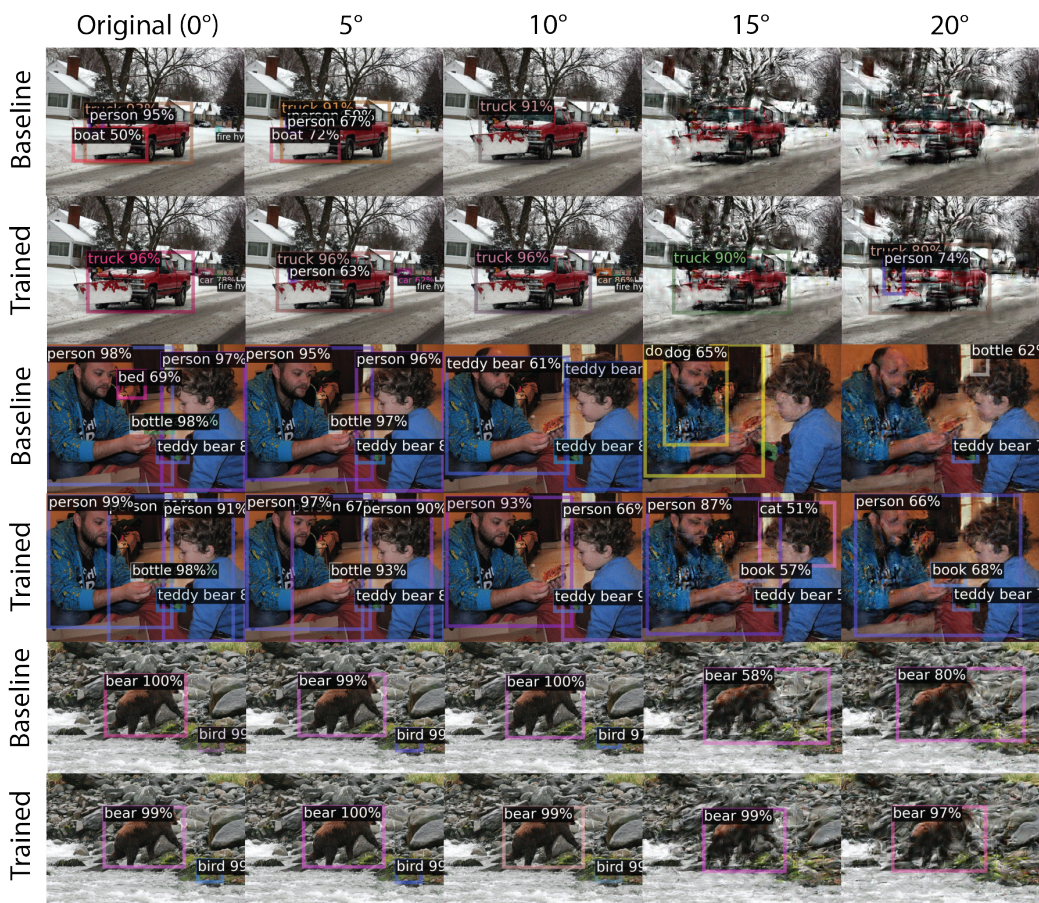
Figure 22: Training improves object detection on Uniform TTM images. Faster-RCNN R50 FPN trained from scratch on peripherally transformed images retains more stable predictions with more accurate bounding boxes as eccentricity increases when compared to the baseline Faster-RCNN R50 FPN model.
