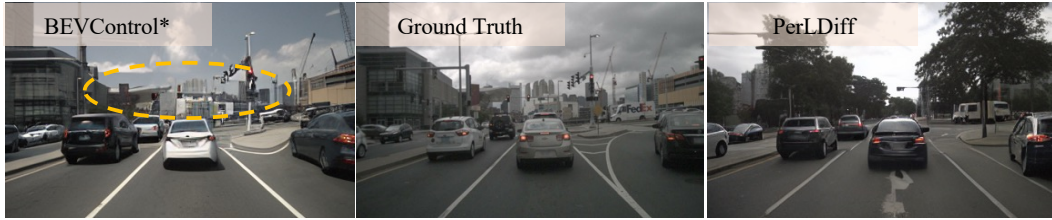
Figure 14: Qualitative visualizations of the generated images reveal discrepancies in background details. As indicated by the yellow circle, PerLDiff produces background elements that do not align with real images due to the incorporation of the PerL masking map.
