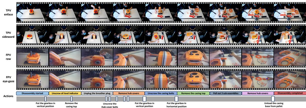
Figure 8: GazeVQA disassembly action includes synchronized multi-view video clips of disassembling the gearbox.
