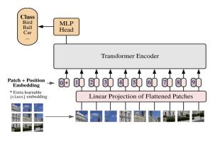
Figure 3: ViT architecture (Dosovitskiy et al., 2020).
