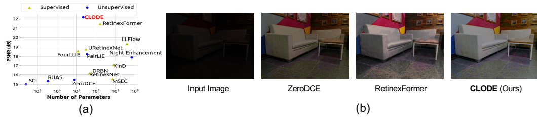
Figure 1: (a) Quantitative Evaluation: The average PSNR values on the LSRW (Hai et al., 2023) and LOL (Chen Wei, 2018), together with the respective parameter numbers for each model. (b) Visual Comparisons with ZeroDCE (Guo et al., 2020) ( unsupervised ), RetinexFormer (Cai et al., 2023) ( supervised ) and proposed CLODE ( unsupervised ).
