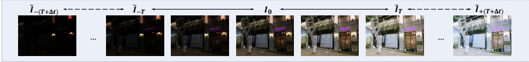
Figure 3: Illustration of User Controllable Design. By manually changing the integration interval from -(T + \Delta t) to +(T + \Delta t) , ours can produce results with different exposure levels.
