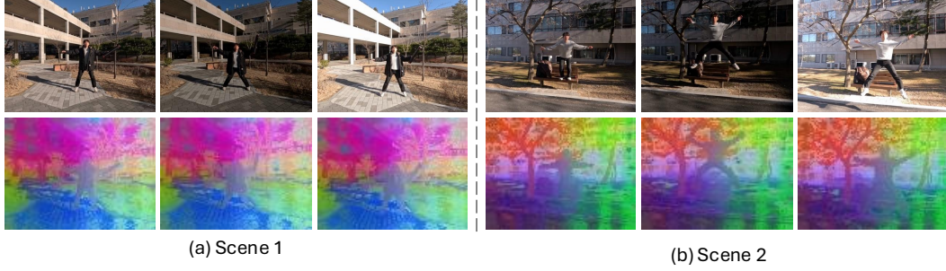
Figure S2: DINOv2 feature visualization under varying exposures. Despite large changes in brightness, DINOv2 embeddings remain consistent, showing robust clustering across different exposure levels.
