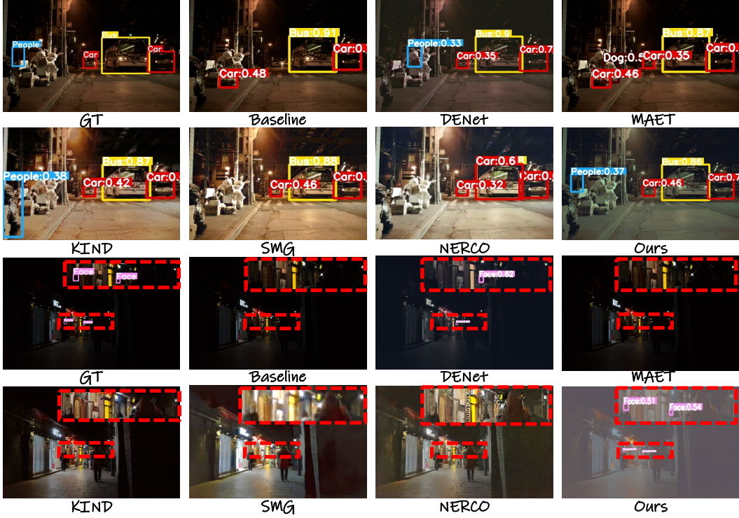
Figure 3: Qualitative comparisons of TOOD detector on both ExDark and UG^2+DARK FACE dataset, where the top 2 rows visualize the detection results from ExDark, and the bottom 2 rows show the results from UG^2+DARK FACE. The images are being replaced with enhanced images generated by LLIE or low-light object methods. Red dash boxes highlight the inconspicuous cases. Zoom in red dash boxes for the best view.
