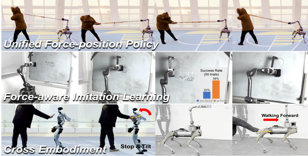
Figure 1: We present a unified force-position policy for legged robots that enables diverse loco-manipulation behaviors, including position tracking, force application, and compliant interactions (top). When used for imitation learning data collection, the policy’s learned internal force estimator provides force-aware demonstrations, improving model performance in contact-rich tasks without external force sensors (middle). Results on quadruped and humanoid robots demonstrate the policy’s versatility and robustness (bottom).
