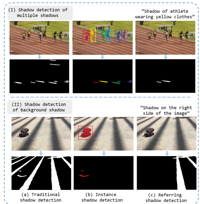
Figure 1: Comparisons of task settings for video shadow detection, instance shadow detection, and our RVSD. Traditional shadow detection (a) segments all shadows, current instance shadow detection (b) detects the foreground objects and segments the associated shadows, while our RVSD (c) can flexibly segment any shadow of interest referred by the text description, including I. those of multiple objects and II. background shadows (objects are invisible in the figure).
