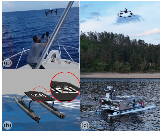
Fig. 1: Illustration of the landing task: (a) manual UAV landing in the real world [3], (b) autonomous landing in simulation under high waves, and (c) the UAV and USV platforms in the real world.
