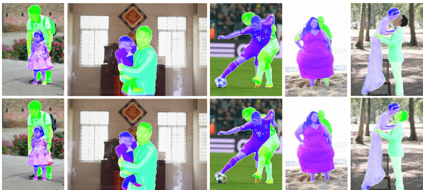
Fig. 6. Subject results on the OCHuman dataset [35] with occluded humans. On the top row are the predictions from the current state-of-the-art model [35]. The results of the proposed framework are shown in the bottom row. It can be seen that occlusions are better handled and background interferences are eliminated.
