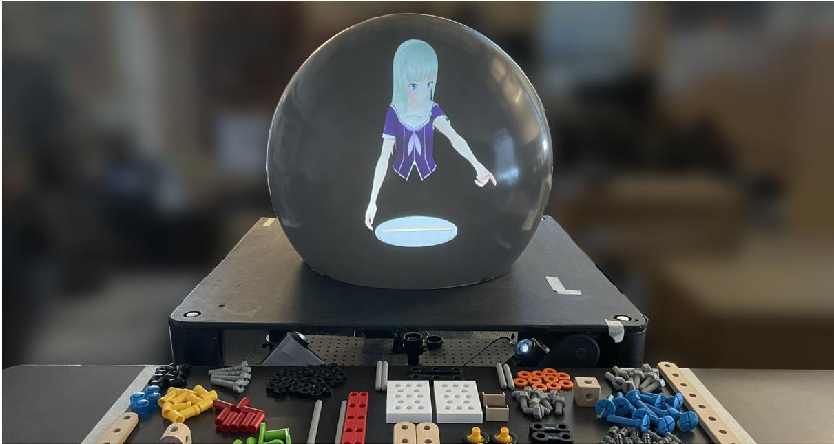
Figure 1: Assembly assistant pointing to real world targets from within a spherical FTVR display.
