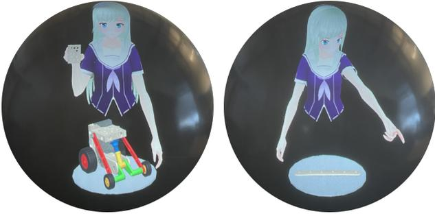
Figure 2: ECA showing a virtual piece (left) and pointing (right) in the spherical FTVR display. The virtual model state is displayed in front of the ECA.
