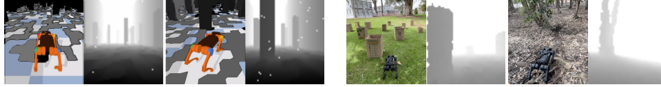
(a) Simulated Environments . For each example, the environment is shown in the left, and the corresponding observation in the right. Aside from the randomized obstacles and terrain, we add randomly placed white spots in the visual observation to simulate the real observation from the depth camera.
