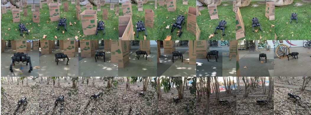
Figure 1: Our method enables quadruped robots to traverse complex environments with obstacles of different shapes in the wild. The learned locomotion policy obtains different agile locomotion skills like flexibly turning before barriers and stably walking on steep lawn, using reinforcement learning. The policy is trained in simulation with our multi-modal delay randomization and deployed in the real-world, unseen scenarios without any adaptation or fine-tuning.
