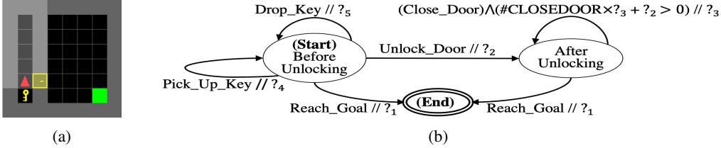
Figure 1: a) A 8x8 DoorKey task; b) The diagram of an SRM designed for the DoorKey task.
