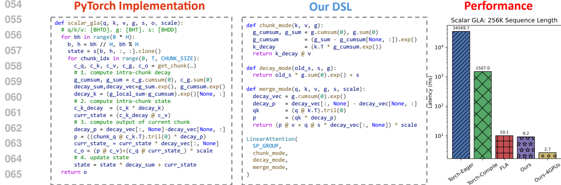
Figure 1: Comparison between PyTorch and our proposed DSL in writing scalar gated linear attention (data type conversion is omitted for simplicity). And the performance comparison of different approaches. Test shape: 32 heads with 128 head dimension. Torch-Eager fails to parallelize the computation, while Torch-Compile also performs poorly. FLA provides expert optimized triton kernels, while program generated by Forge offers comparable performance to handwritten kernels with the scalability to distributed environments.
