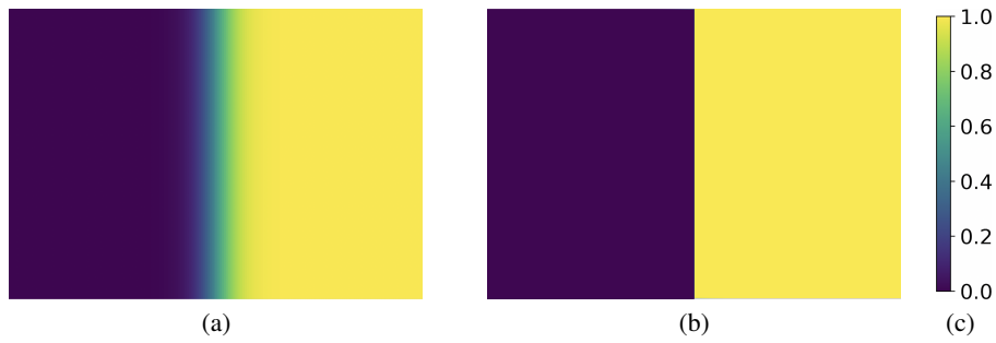
Figure 2: (a) shows the conditional probability that a point is drawn from each Gaussian. (b) shows the most likely class given any data point. (c) shows the mapping between color and class probability.
