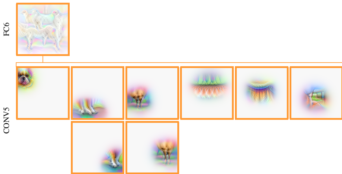
Figure 16: Side dogs . The visualization for the FC6 nodes resembles animals from side view, a typical image positioning for dogs. In the images generated for associated units in the convolutional layer, we see how the network uses different filters to put this pattern together. The first depicted filter captures a dog head, typically found at the top left part of the image. The second and third filters focus on the legs. In the third row, we can see that other units for these filters are also commonly activated with the feature, showing that there are typical positions for legs in both the left and right lower parts of the image. In the last three prototypes, we recognize horizontal lines, which overall resembles the typical shape and position in the image where we would expect the back of an animal.
