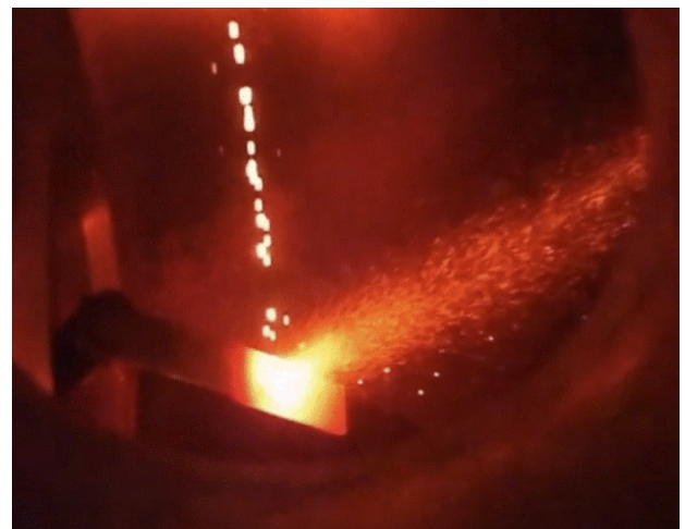
Fig. 2: A metal alloy ultrasonic atomizer creates additive-manufacturing friendly powders by turning inductively heated molten metal into spherical droplets via ultrasonic vibration.
