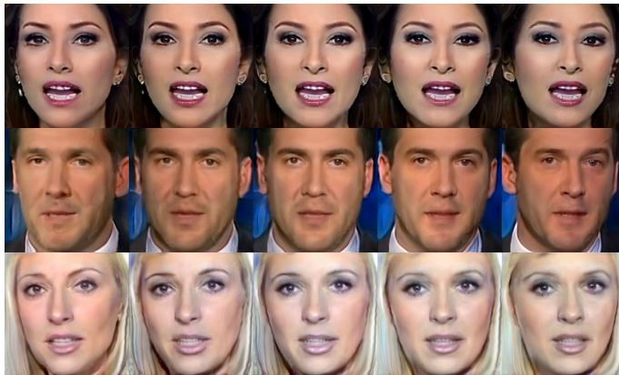
Figure 12: FFHQ and FaceForensics simultaneous training results. We show qualitative results of our model simultaneously trained on FFHQ and FaceForensics, rendered from five different cameras (columns) for three identities (rows). We observe lower view-consistency compared to our model only pre-trained on FFHQ.
