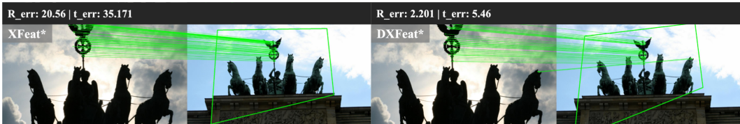
Figure 2: Compares XFeat*(left) with DXFeat*(right). We observed that DXFeat* provides more reliable keypoints compared to XFeat*, resulting in significantly smaller rotational and translational errors. The green square grid represents the camera viewpoint projected back after the perspective transformation, highlighting DXFeat*'s superior accuracy and robustness in feature matching.
