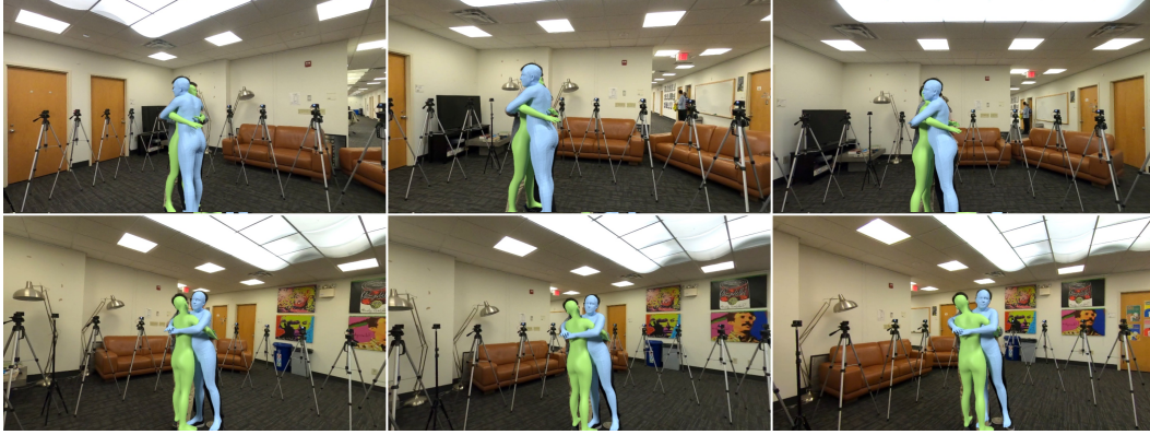
Figure 8: Harmony4D ground-truth mesh visualized from six camera views for the hugging sequence.
