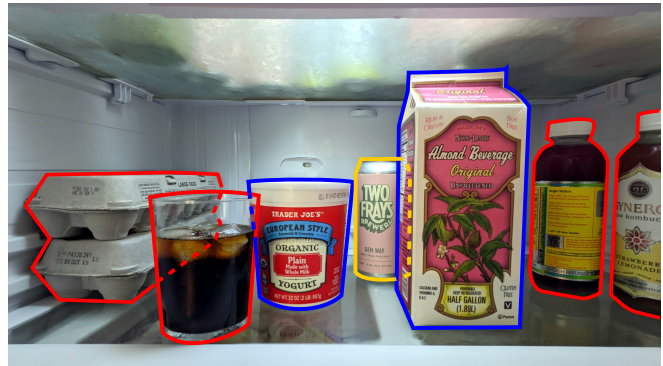
Fig. 1. An example MAMO problem to retrieve the beer can (object-of-interest or OoI, yellow outline). The yogurt and almond beverage are movable objects (blue outlines). All other objects in the scene are immovable obstacles (red outline).
