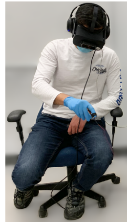
Figure 5: A participant interacting with a virtual object while wearing the VR headset with the Leap Motion hand tracker, VCA and nose-canceling headphones.
