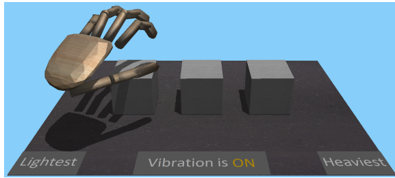
Figure 7: Three virtual cubes with random weights are placed in front of the participant to sort in ascending order from left to right. The "Vibration On" label indicates to the participant that they should expect vibration from the voice-coil actuator when picking up objects.
