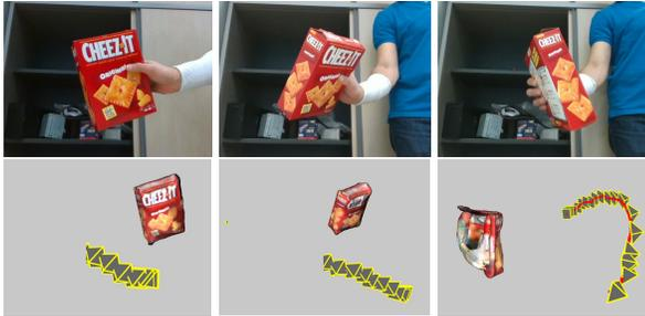
Figure 7. **Incremental reconstruction and pose tracking is prone to fail beyond the segment boundary.** On this representative example, the incremental reconstruction and pose tracking procedure works well as long as the front face is visible. When the front face starts to disappear and new parts start to appear (last column), reconstruction degrades and pose tracking drifts.
