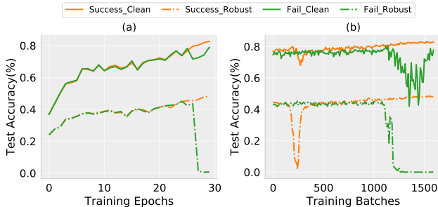
Figure 2: Comparison of a success mode (orange) and a failure mode (green) of fast adversarial training for 30 epochs. In plot (a), we show the test clean and robust accuracy for each epoch. In plot (b), we report the same quantities for every 10 batches for the last 5 epochs. Both models encounter catastrophic overfitting, but only the model in the failure mode never recovers.
