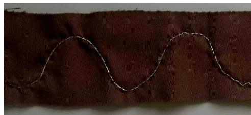
Fig 1 Conductive yarn embroidered onto the fabric to form a piezoresistive strain gauge.
