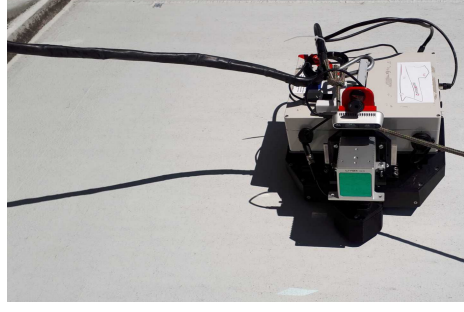
Figure 1: Example of tethered robot used to clean industrial surfaces in H2020 project BugWright2.
