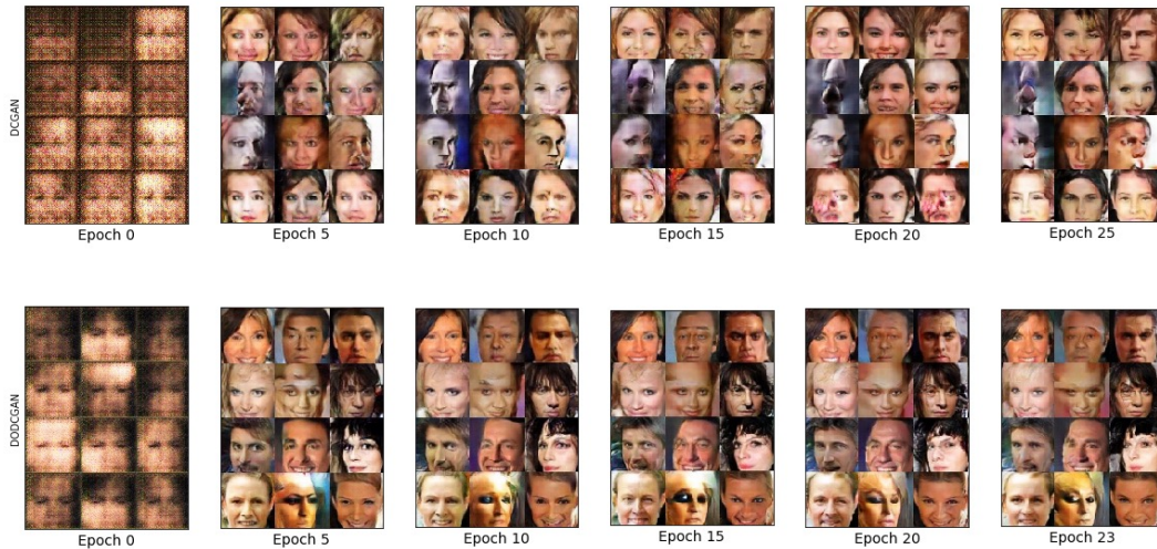
Figure 10: Training images with fixed noise for DCGAN and DO-DCGAN until termination.
