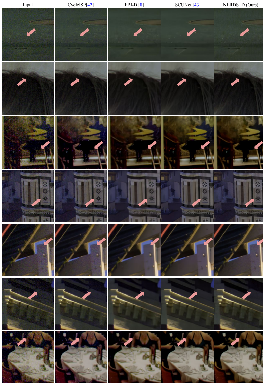
Figure 12: Qualitative results on MIT-Adobe FiveK. CycleISP often fails to remove noise, while FBI-D and SCUNet over-smooth or over-sharpen images. Note that NERDS+D uses only 5 test noisy images and estimated noise parameters from them for training. ( Zooming-in for the best view. ) We use T of NERDS to convert raw images denoised by FBI-D to RGB images.
