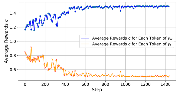
Figure 4: The curve of changes in self-calibrated rewards for positive and negative samples over training steps, with a sample point taken every 10 steps.
