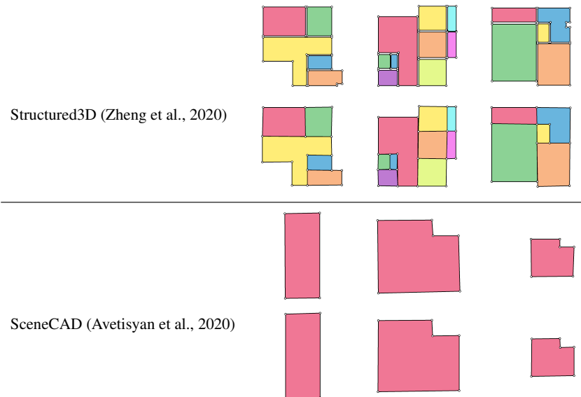
Figure 8: Qualitative examples of indoor floorplans predicted by Pix2Plan on the Structured3D (Zheng et al., 2020) test set and the SceneCAD (Avetisyan et al., 2020) validation set. For each dataset, the first row depicts the ground truth indoor floorplan and the second row showcases Pix2Plan’s floorplan predictions. Pix2Plan is able to consistently predict accurate indoor floorplans in a tight-layout.
