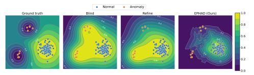
Figure 1: DeepSVDD trained on 2D synthetic contaminated training data with different configurations: (I) Supervised AD with ground truth labels for reference, (ii) "Blind" considering all samples as normal, (iii) "Refine" filtering out a fraction of the anomalies, and (iv) EPHAD updating the "Blind" anomaly detector using evidence computed on the samples available at test-time.
