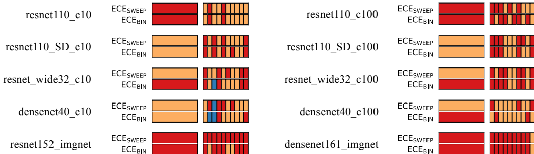
Figure 2: Bias affects which recalibration algorithm is preferred. For ten models, we report which recalibration method is determined to be superior based either on ECE_{\text{BIN}} or ECE_{\text{SWEEP}} . The wide bar indicates the superior method using entire validation set (mean of X instances); narrow bars each use a random sample of 10% of the original validation set. Recalibration methods tested are histogram binning , temperature scaling , and isotonic regression .
