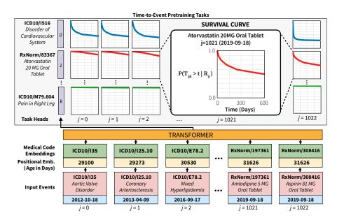
Figure 1: MOTOR architecture and TTE pretraining tasks, as applied to a patient. Note how tasks (survival curves) vary at each time step j, e.g., atorvastatin risk increases given a history of cardiovascular disorders.
