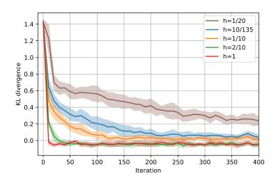
Figure 5: Convergence of KL divergence for different step sizes h, with all other parameters set as Ours in Table 1. Each curve shows the mean over 10 random seeds, with shaded areas indicating variances. Larger step sizes lead to faster convergence.
