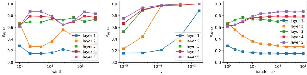
Figure 16: The effect of the width, weight decay  $\gamma$ , and batch size on the alignment for a fully connected network. The training proceeds for  $10^5$  iterations, when the training stops decreasing significantly. The training proceeds with **SGD**.
