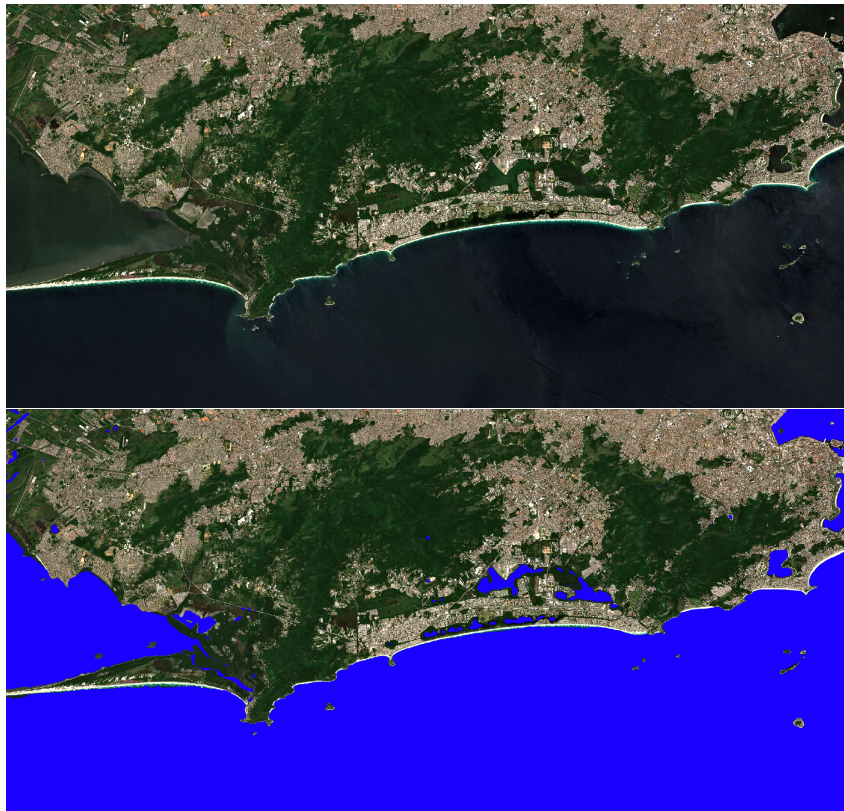
Figure 1: Earth Surface Water trained model predictions (blue) on a Sentinel-2 scene captured over Rio de Janeiro, Brazil.
