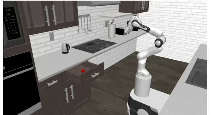
Fig. 9: Our RoboCasa simulation setup includes a 7-DOF Franka Emika Panda arm with a 2-fingered gripper.
