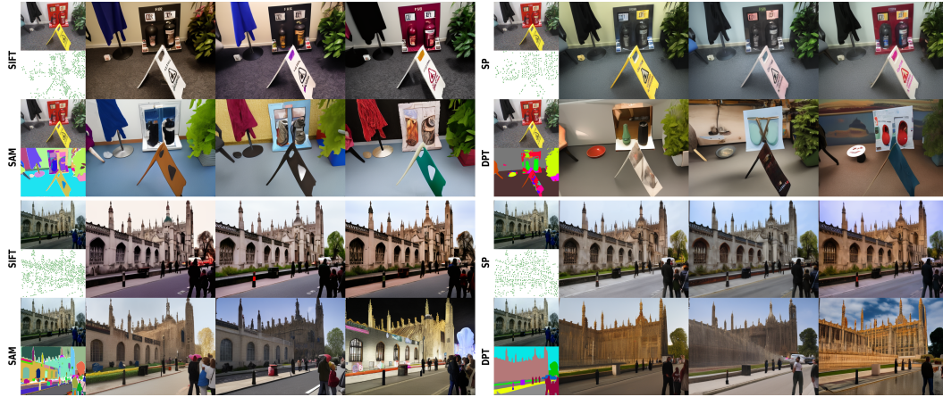
Figure 2: Reconstruction output for different seed and similar conditioning. Visualization of SIFT/SuperPoint/DPT/SAM2 conditioning. The ground truth image is displayed on the top left and the conditioning is displayed on the bottom left. As opposed to segmentations, SIFT/Superpoint display low variability under different seeds.
