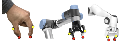
Figure 2: 4 finger keypoints used as tracking points for robots with parallel-jaw grippers.
