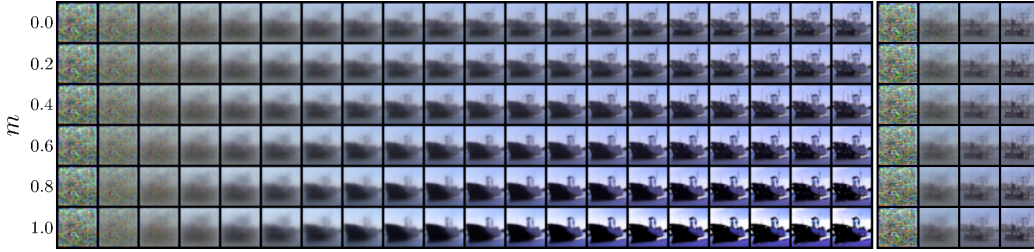
Figure 4: Ensemble denoising predictions \bar{x}_0^{1:T} in 20-step (left) and 4-step (right) iDDIM sampling process with varying m .
